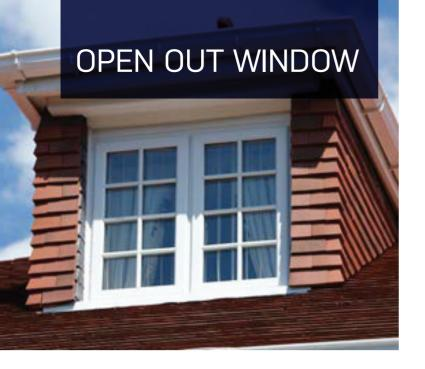
This window may be opened outwards with its friction hinges holding it in a desired position. Locking is achieved by the mushroom cams and/or the shootbolt pins of the locking mechanism, fitted to the opening edge of the window, engaging into the keeps fitted to the outer frame.
