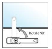
Turn key to unlock. Rotate handle 90° to vertical, open slightly and close handle to engage night vent slots.
