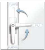
Note: The window must always be fully shut before changing the handle position.
