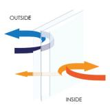
Although a double glazed window is capable of retaining far more internal heat, the less efficient types allow a certain amount to pass through the air space and thus warm up the outer pane. This would not therefore allow condensation to form on either pane.
