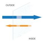
A single glazed window cannot retain heat within the room and the lower temperature of the glass allows the moisture in the air to condense on the cold surface. This is often more evident in rooms in which there is a lack of ventilation.
