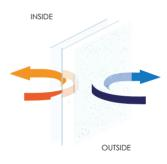
The new generation of thermally efficient double and triple glazed windows allow little or no heat through to warm up the outer pane. This creates the condition which allows condensation to form on the outside surface of the
